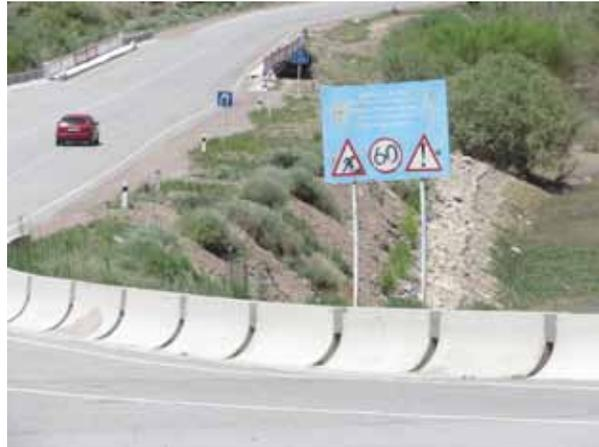
Road work signs should comply with national standards for color, shape, and symbols. The six-zone approach puts signs to effective use in positions where their message is most needed.
