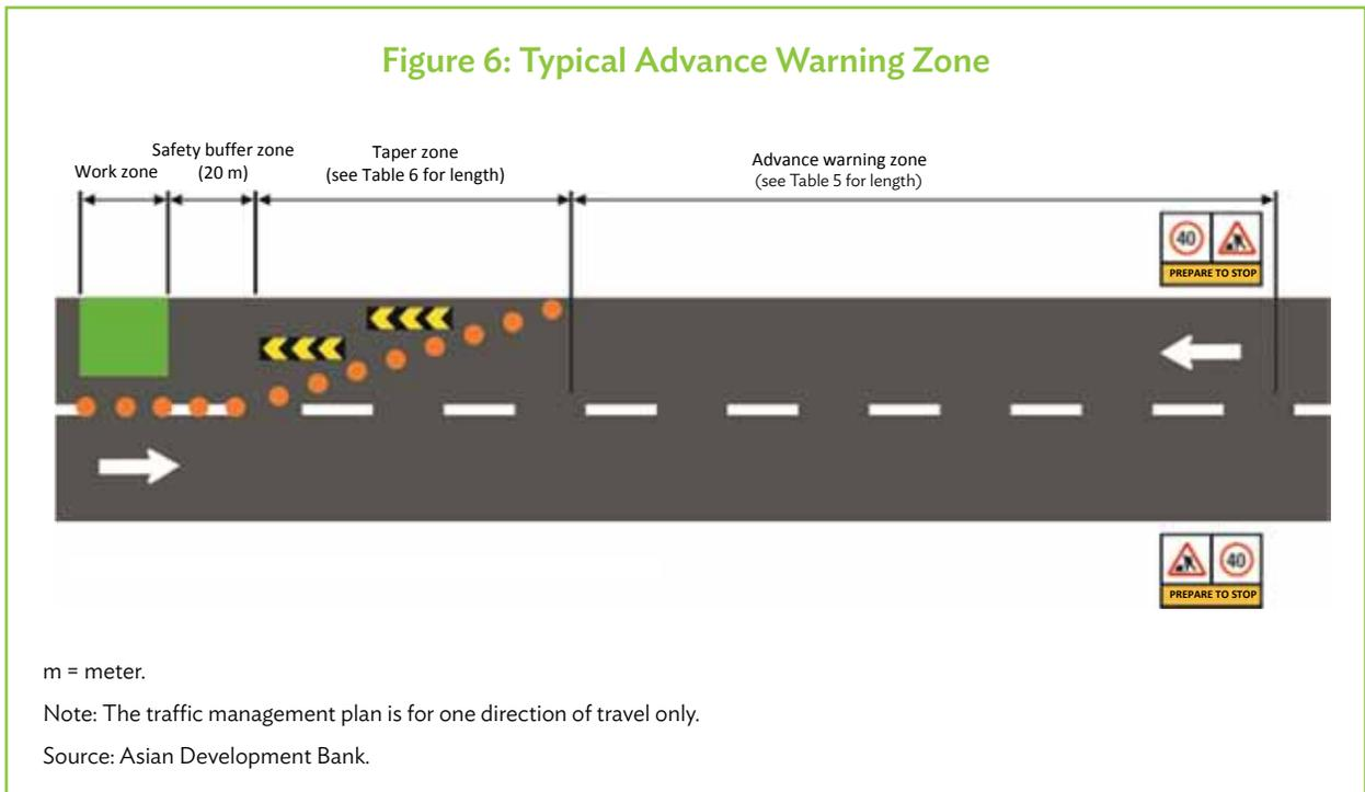
83. Advance warning of road worksites creates an expectation of changed traffic arrangements so drivers and riders can modify their driving or riding and look for appropriate guidance. The advance warning signs should be obvious, and the layout of the worksite management scheme should be clear and definite, allowing only one course of action from the driver and/or rider.
