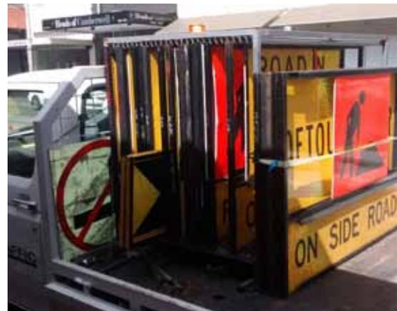
Simple frames can be constructed to carry the multimessage signs to and from the worksite in a small truck or van.
