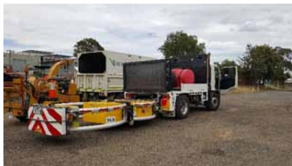
Truck-mounted attenuators provide physical protection for workers at road worksites, where the provision of safety barriers or road closures is not practicable.
