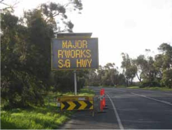
An example of a trailer-mounted variable message sign located just off the shoulder of a rural highway with a speed limit of 100 kilometers per hour (driving on the left side).
